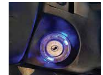
White Illumination Facia and Ignition Switches for Driver guidance in Night
