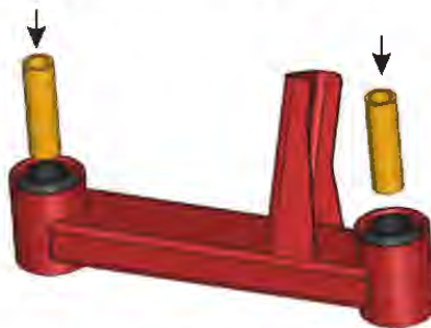
Fig. 9.14 Insert Inner metal sleeve into rubber bushes
