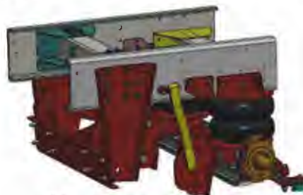
Fig. 9.15 Put Top Beam Assembly with new wear pad
