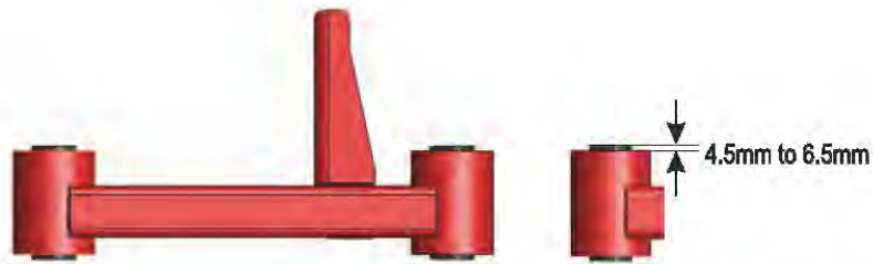
Fig. 9.13 Check the height of rubber bush face to beam tube face within 4.5 to 6.5 mm
