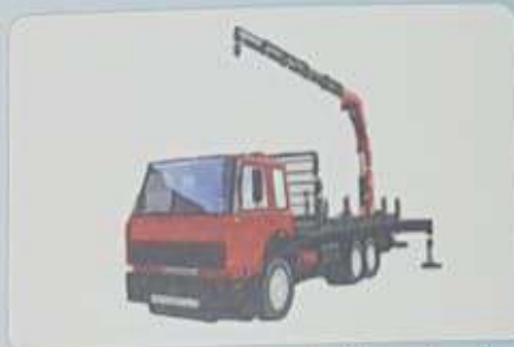
Truck Mounted Crane
