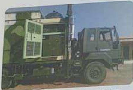
Mobile Power Generator
