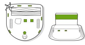
**Important:** Do not spray cleaning solution or water onto the sensors or sensor openings.
