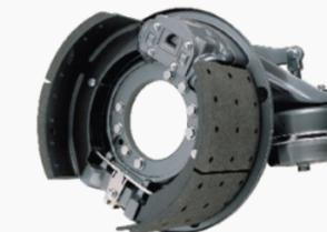
Full Air S cam Brakes with Auto slack Adjuster & ABS, Brake drum diameter - 360mm
