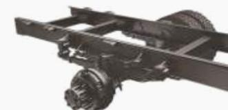
Depth - 223mm, Flange Width - 60mm, Thickness - 7mm (Ladder type heavy duty frame with Riveted/boted cross members)
