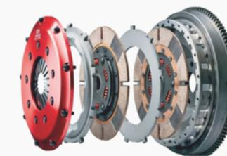
330mm Single plate dry friction type Low hysteresis clutch with high size clutch Booster to reduce the clutching efforts
