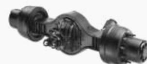
Front Axle - Heavy duty forged I beam, reverse elloit type
